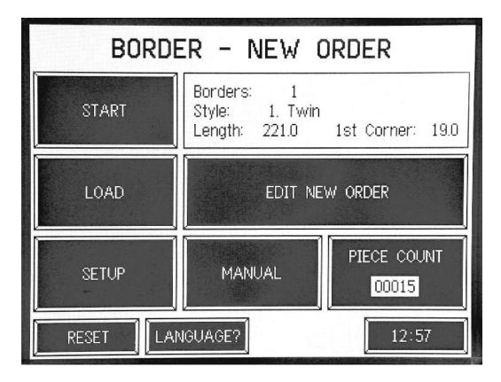
This is the main screen. Pressing START will run the machine in automatic. The top right display box shows how many borders will be made continuously after the START button is pressed. The LOAD button raises the foot, puller, and measuring wheel for loading. Pressing the LOAD button brings up another screen:
