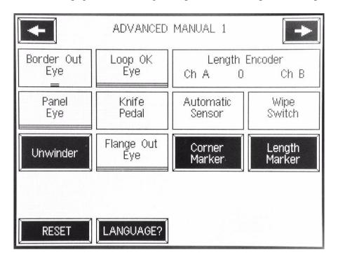
The inputs are represented by plain boxes with small "hash marks" or "bars" at the bottom. The bars and marks indicate whether the input is on or off. The "3 dimensional" looking rectangles are buttons and represent outputs. A dark background indicates the output is off. Pressing the button will turn the output on or off. Some outputs toggle on/off, others must be held down to stay on. There are 3 screens that show all of the machines inputs and outputs.
