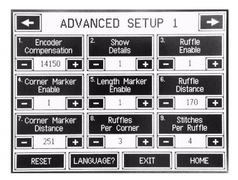
This screen displays the internal machine settings that control all functions. The number in the upper left corner of each button represents the counter/setting number and is used on the SHOW ALL SETTINGS page matrix. Notice that the RUFFLE ENABLE setting is the same setting as the RUFFLE ENABLE button on SETUP BORDER MODE page 2 mentioned earlier. The same is true for many of the other settings shown.
