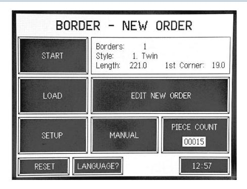
Press MANUAL to access the manual run page and enable the foot switches for manual sewing and foot lift functions. You can turn on the ruffle cycle for testing and access the advanced manual pages for testing inputs and outputs.
