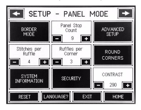
This screen has an additional button for adjusting the PANEL STOP COUNT that controls where the panel stops for turning the corners and a ROUND CORNER button for selecting the corner mode. When the ROUND CORNER button has a WHITE background the machine is in the ROUND CORNER mode. When the background is DARK the machine is in the STRAIGHT CORNER mode.
